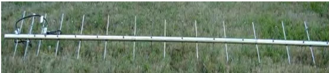
Figure 6. 450 MHz Antenna
