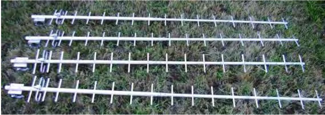
Figure 7. 915 MHz antenna
